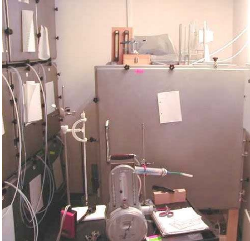
Figure 2 Climatic chambers: one 1 m 3 chamber to the right and several 320 litre chambers to the left
