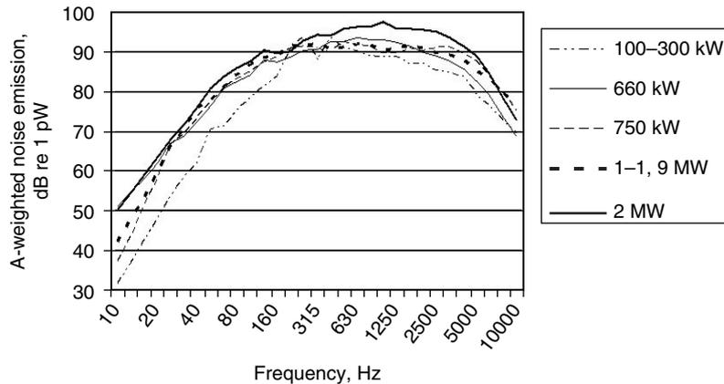
Figure 3. A-weighted spectra of wind turbine noise in 5 different classes of turbine nominal power. From [15]
