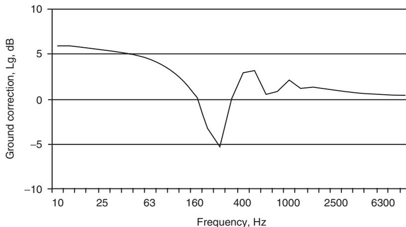
Figure 1. Illustration of ground correction. Source height 80 m, receiver height 1.5 m and 500 m distance; propagation over porous ground and 8 m/s wind speed.
